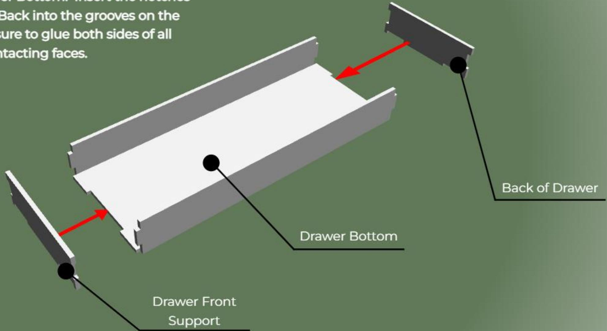
Glue the Front of Drawer to the Drawer Front Support. The bottom should be flush with the bottom of the drawer but centered on the otherwise.
