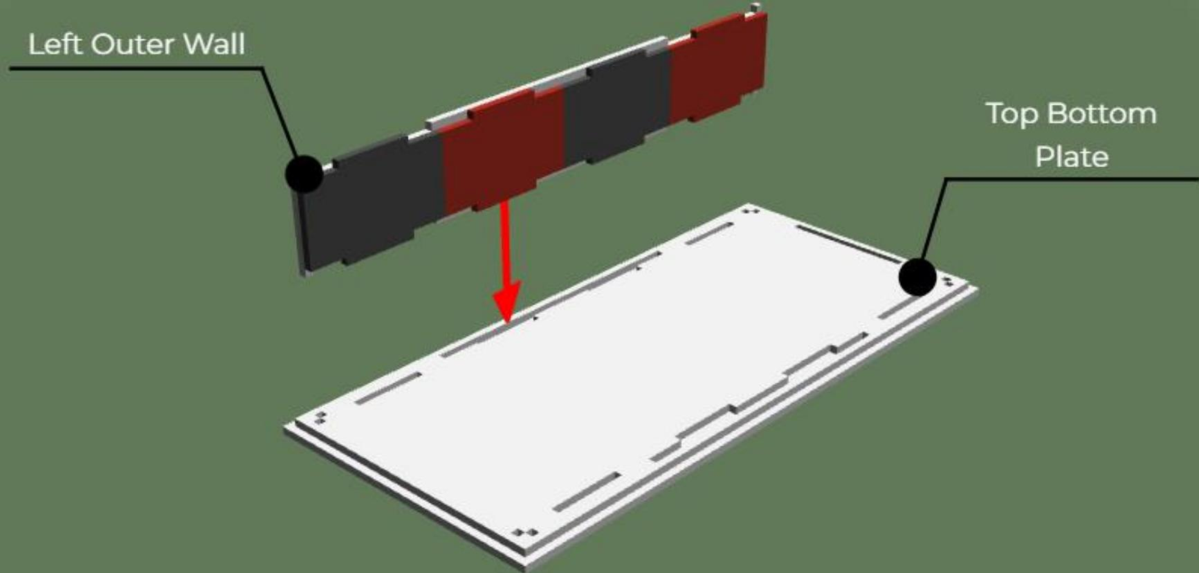
Insert the notches on the Left Outer Wall Assembly to the grooves on Top Bottom Plate. Glue both sides of all contacting faces.
