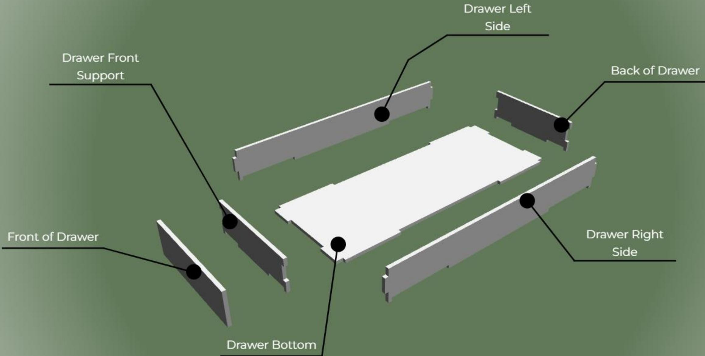
Glue the Left Side and Right Side of the Drawers to the Drawer Bottom. Be sure that the notches on the bottom are inserted into the grooves on the side and glue both sides of all contacting faces.
