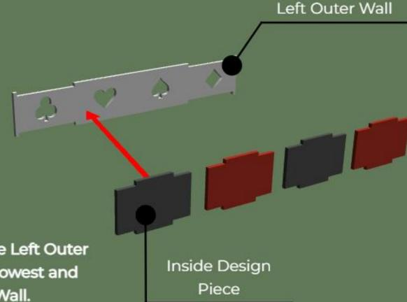
Glue the Inside Design Piece to the Left Outer Wall. They should align with the lowest and highest parts of the Outer Wall.
