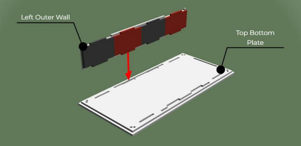
Insert the notches on the Left Outer Wall Assembly to the grooves on Top Bottom Plate. Glue both sides of all contacting faces.
