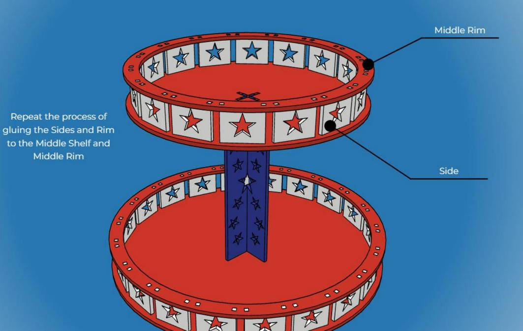
Repeat the process of gluing the uprights together and gluing them to the Middle Shelf.
