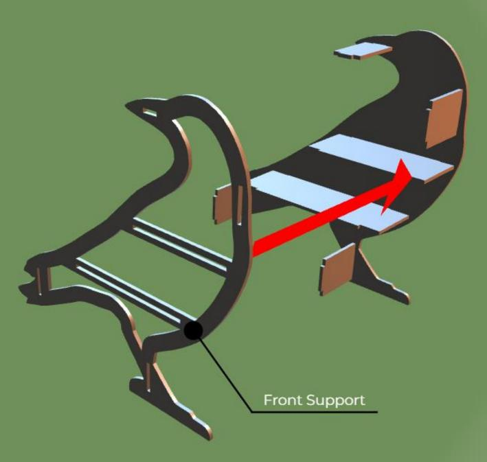
Glue the Front Face onto the Front Support (if you want). This piece is meant to hide the joinery from the shelves and isn't necessary if you don't want to use the material.
