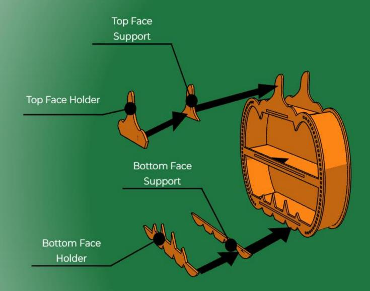
Glue the Top Face Support the the Front and then glue the Top Face Holder to the Top Face Support.
