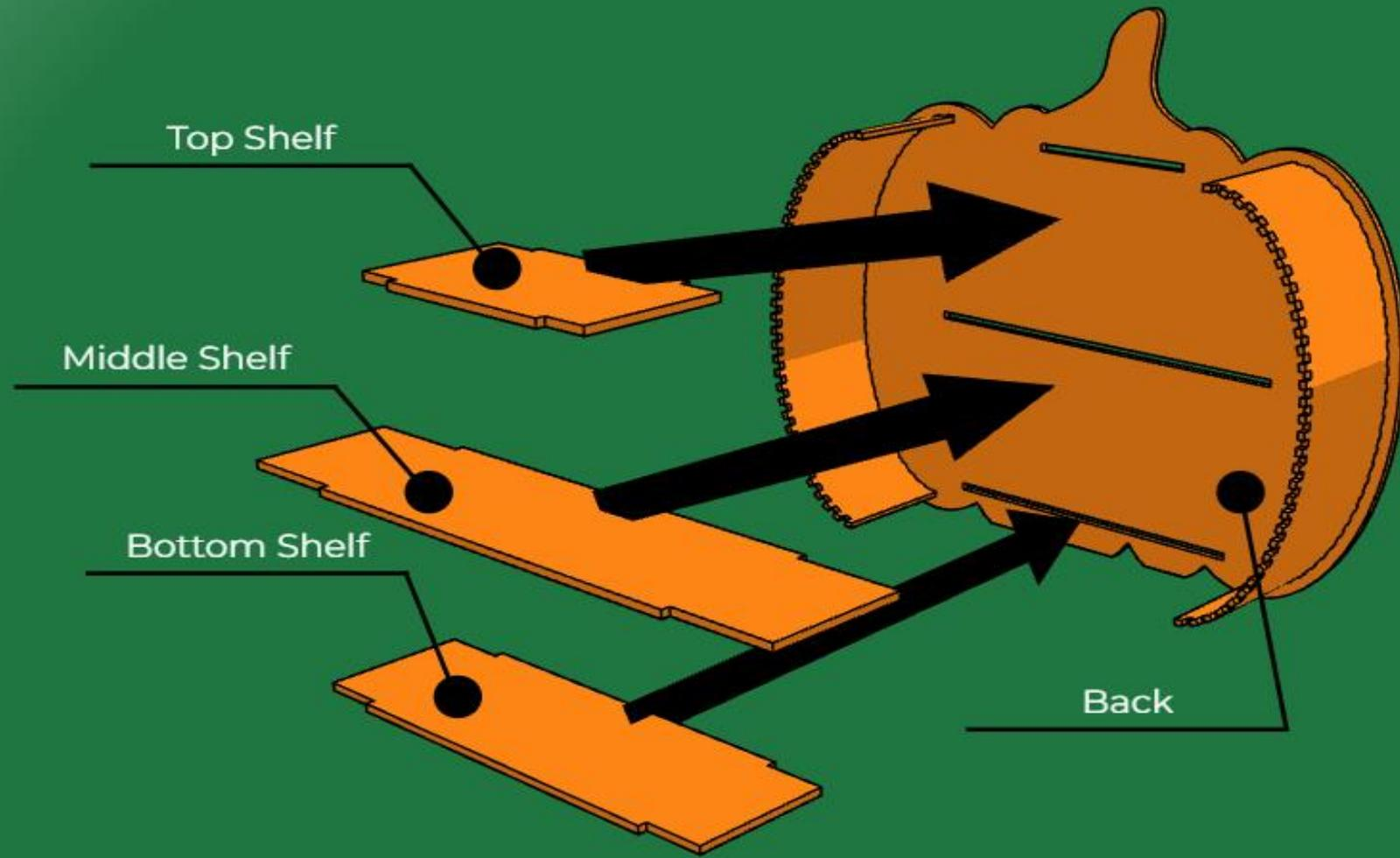
Insert the tabs on the Top, Middle, and Bottom Shelf into the notches on the Back. Glue both sides of all contacting surfaces.
