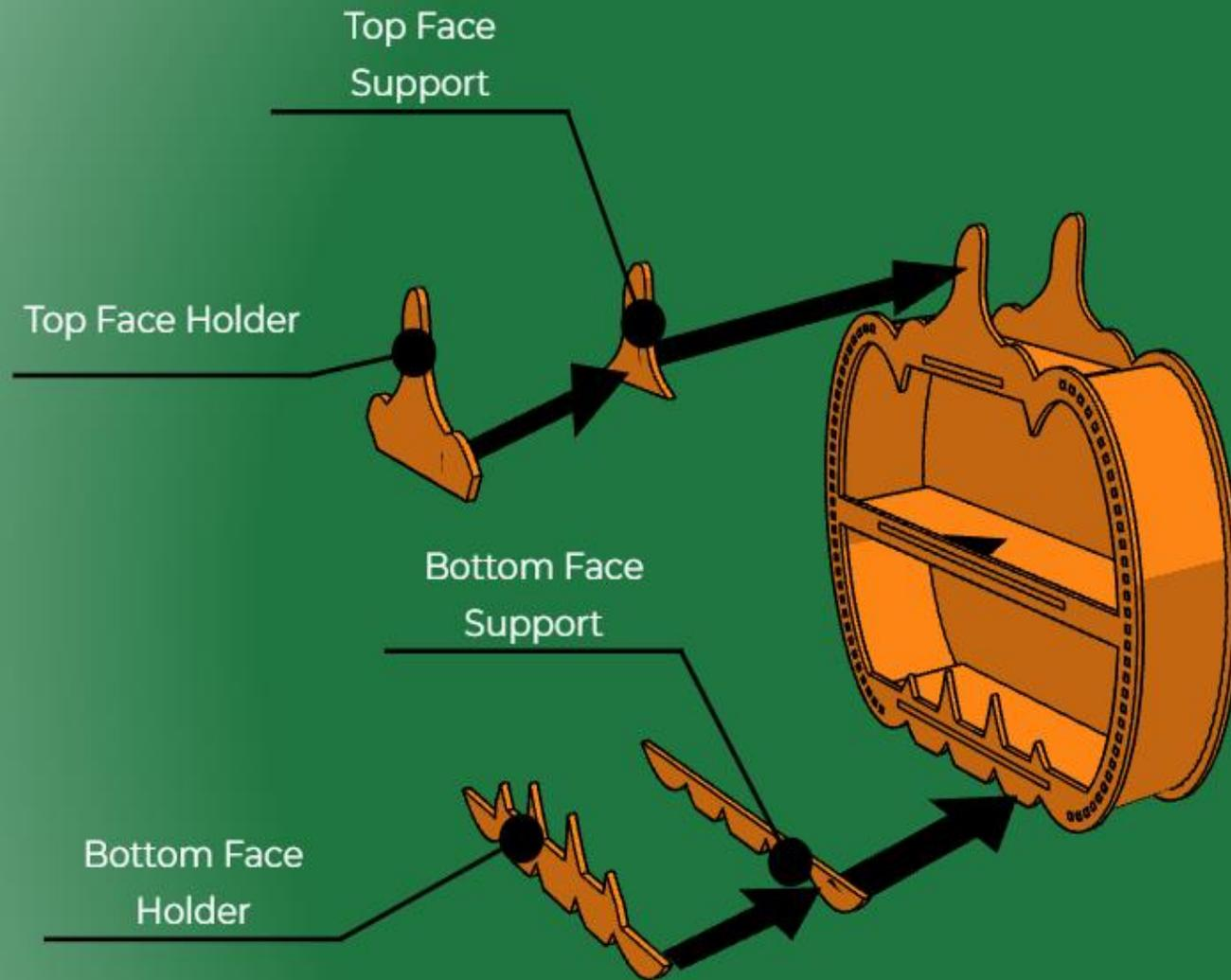
Glue the Top Face Support to the Front and then glue the Top Face Holder to the Top Face Support.
