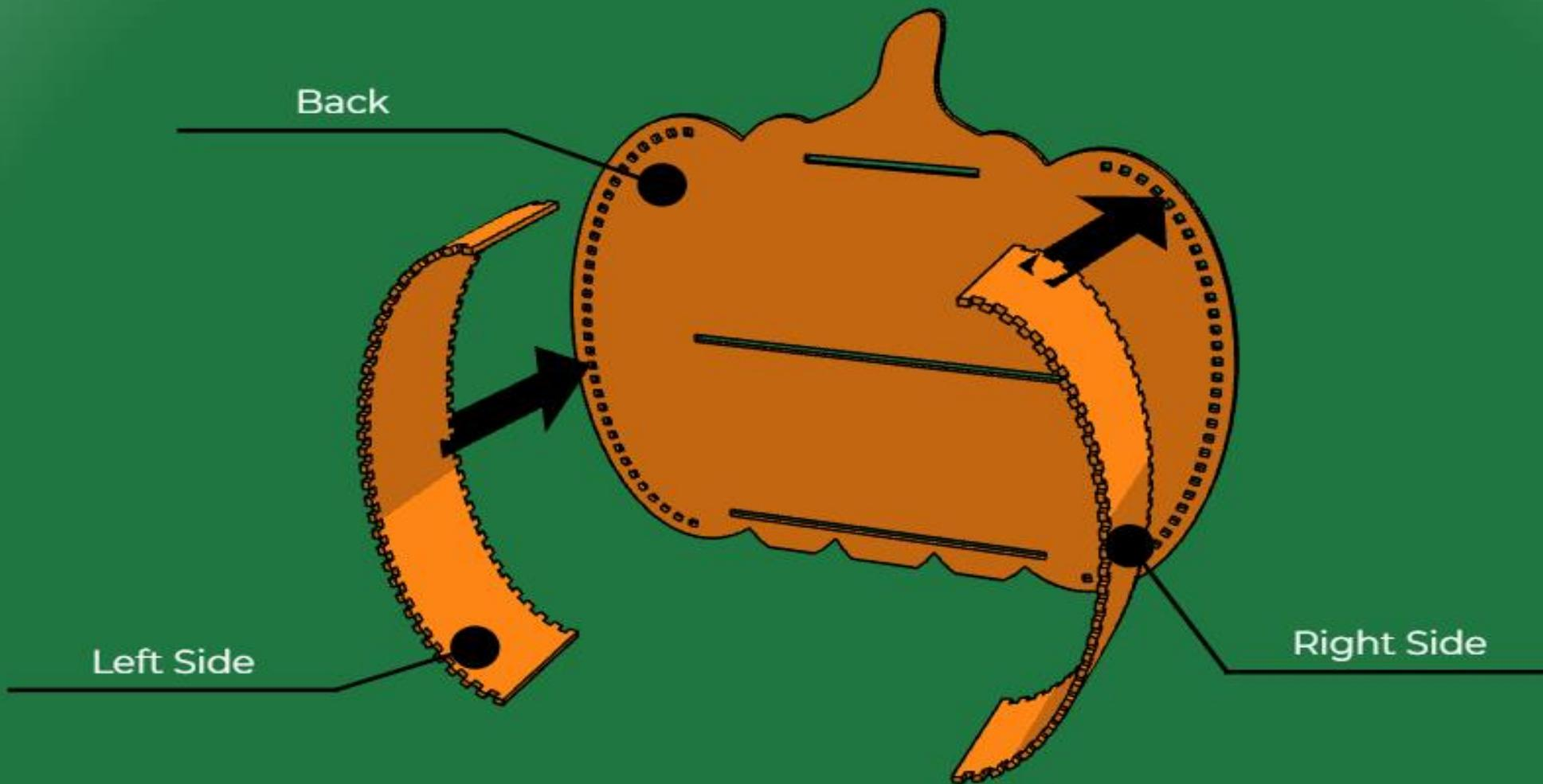
Insert the tabs on the sides into the notches on the back. This will require careful bending and some stretching of the sides. Glue both sides of all contacting faces.
