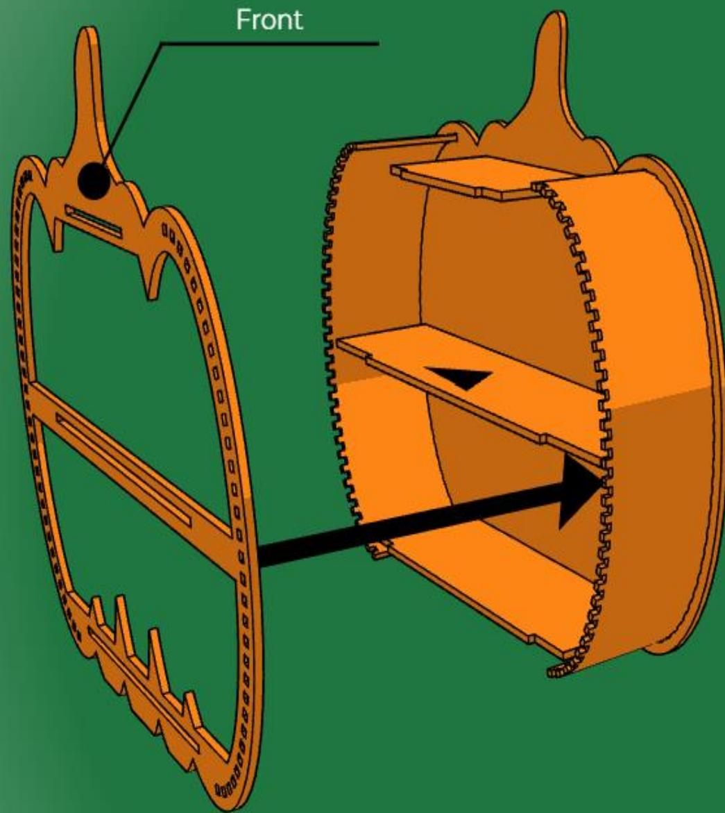
Attach the Front by inserting the tabs on the Sides and Shelves into the grooves on the Front.
